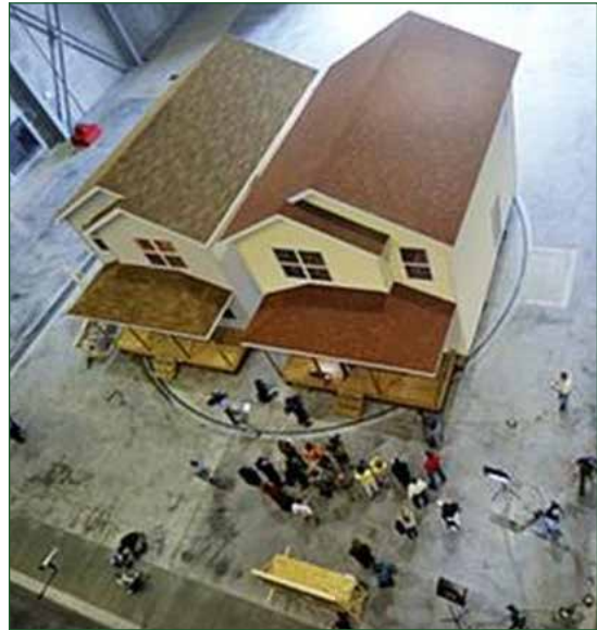
IBHS Research Center's wind tunnel test facility.
