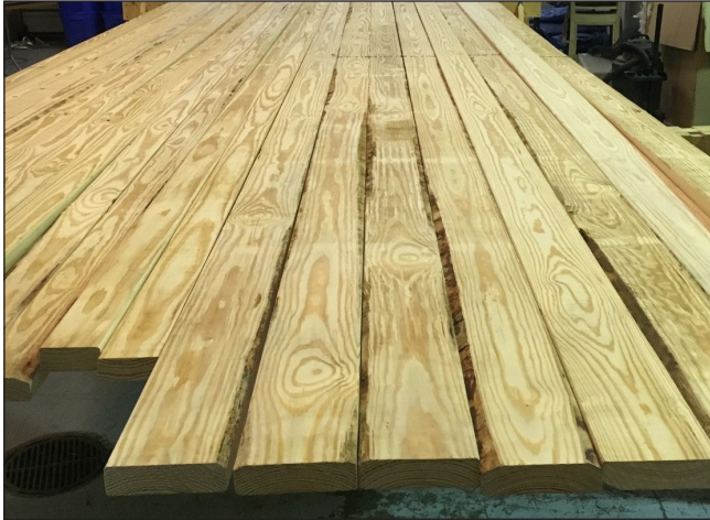
16- and 20-ft-long pine lumber with minimal strength-reducing characteristics that will be used to develop the initial clean wave signatures.
