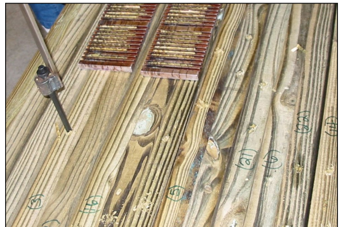
Figure 2. Retention in charges of treated lumber is determined by removing increment cores and combining them for chemical analysis.
