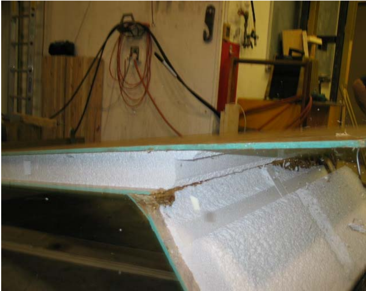
FIGURE D3. AXIAL LOAD (COMPRESSION) TEST (Shear failure through foam propagated from horizontal electrical chase at bottom edge of panel)
