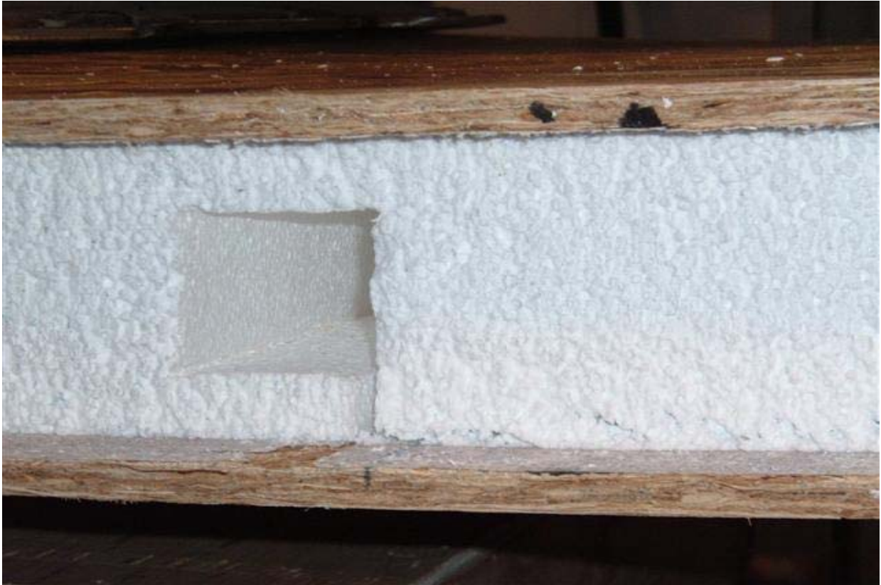
FIGURE D4. TRANSVERSE LOAD TEST (Failure on tension side at electrical chase holes)
