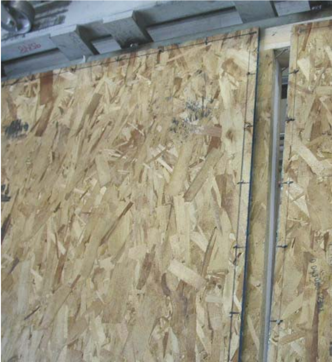
FIGURE D1. RACKING SHEAR TEST FAILURE (Nails tear away from center spline)
