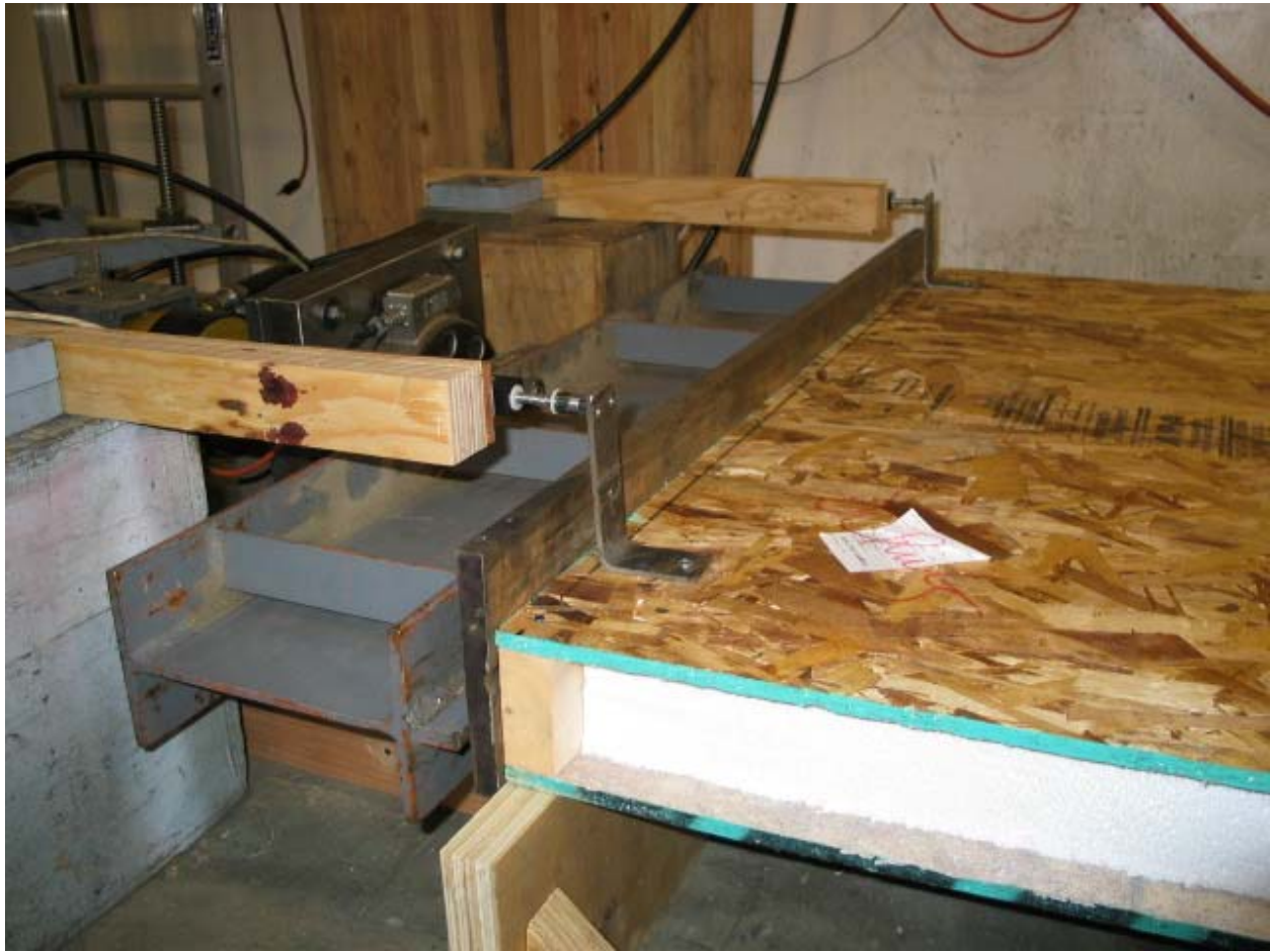
FIGURE C4. AXIAL (COMPRESSION) LOAD TEST ASSEMBLY – LOAD HEAD WITH INSTRUMENTATION
