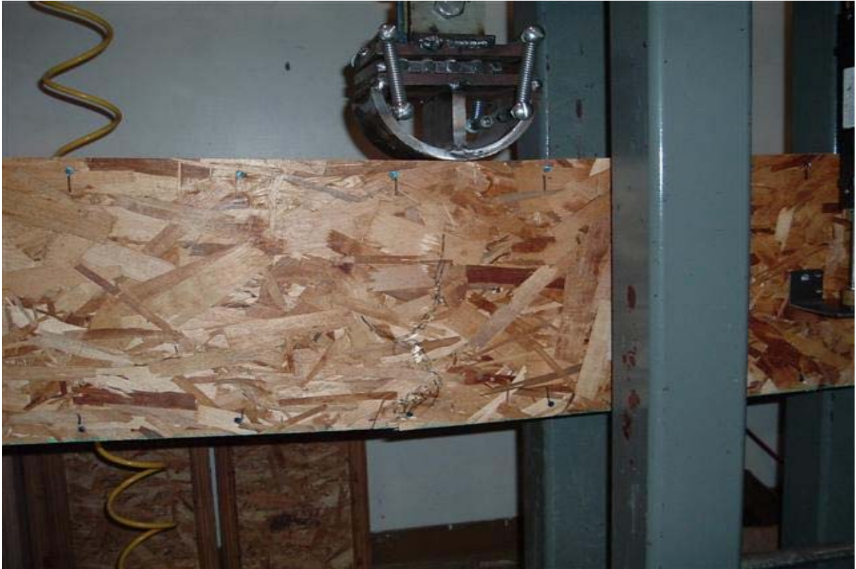
FIGURE D5. LINTEL BENDING TEST (Tension failure of OSB skins at one-of-two load points)
