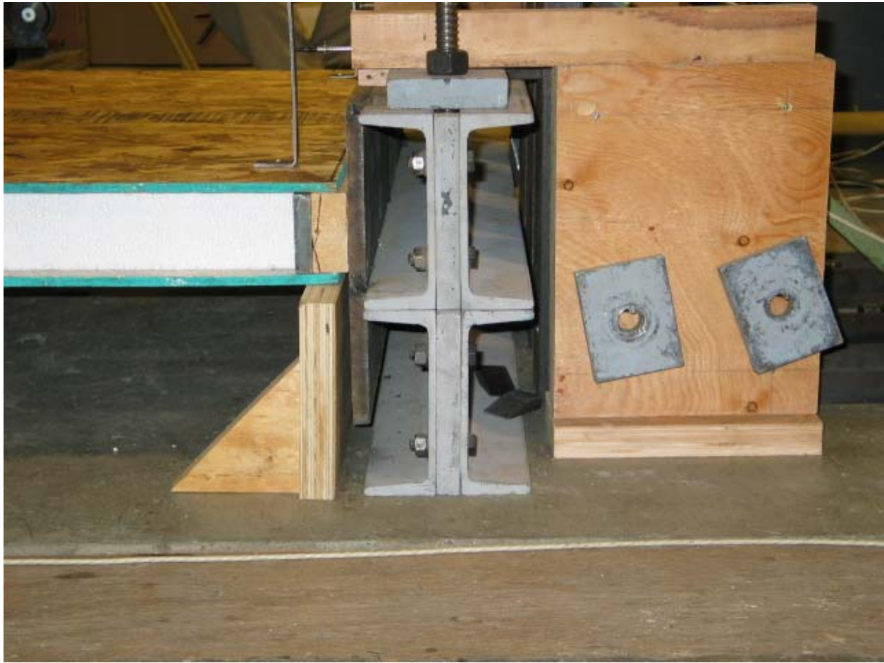
FIGURE C5. AXIAL (COMPRESSION) LOAD TEST ASSEMBLY – REACTION BEAM
