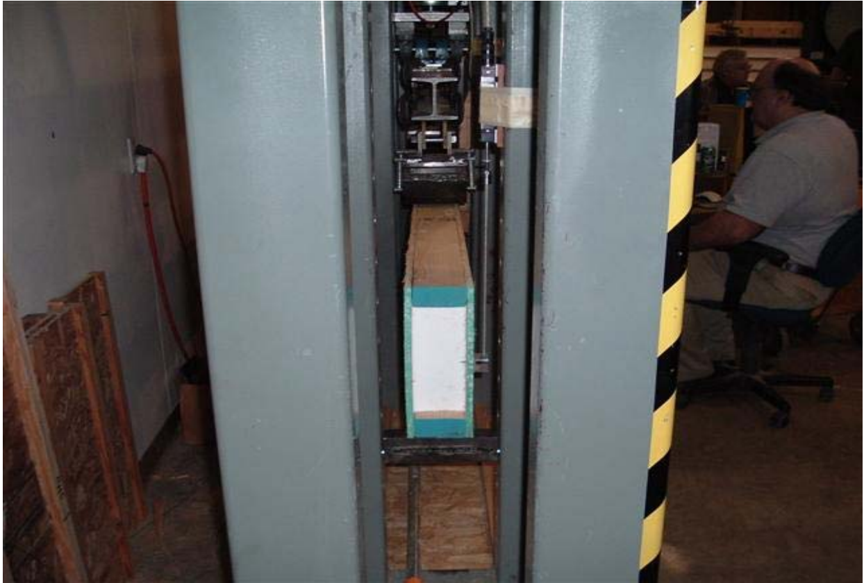
FIGURE C11. LINTEL LOAD TEST ASSEMBLY – END VIEW
