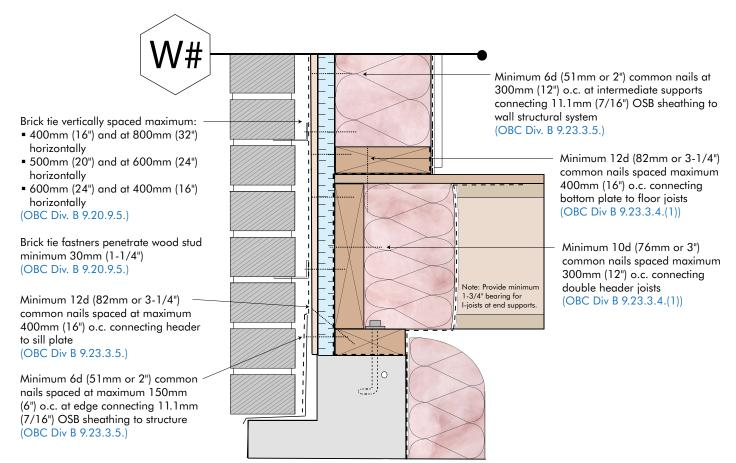
Note: Provide proper gap between wood structural panel and concrete as per local code requirements and manufacturer recommendations.
