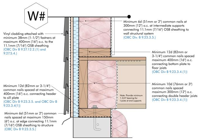
Note: Provide proper gap between wood structural panel and concrete as per local code requirements and manufacturer recommendations.
